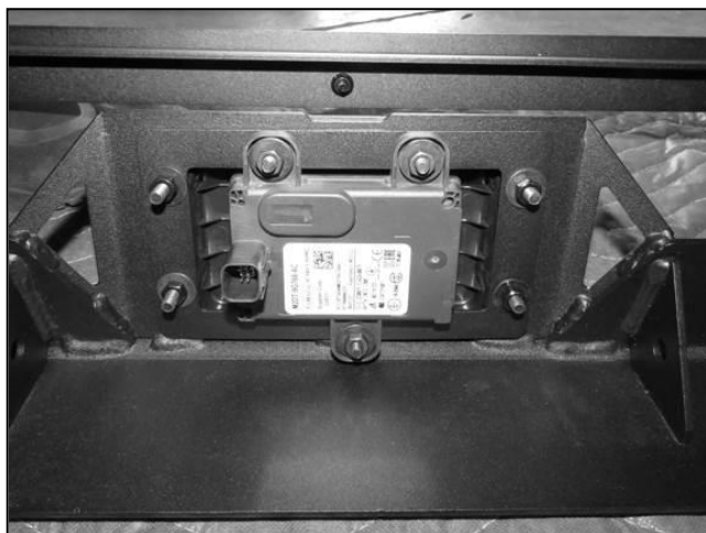
(Fig 17) ACC sensor assembly attached to back of Bumper
