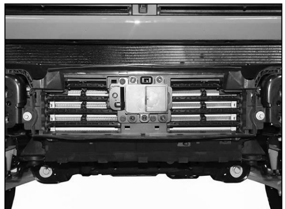
(Fig 5) Remove the shutter assembly. Models with ACC sensor (pictured), unplug and remove sensor from shutter
