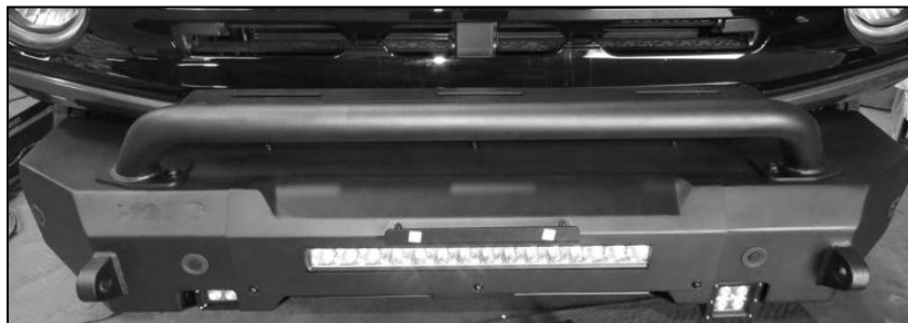
(Fig 32) Reinstall center Cover Plate
