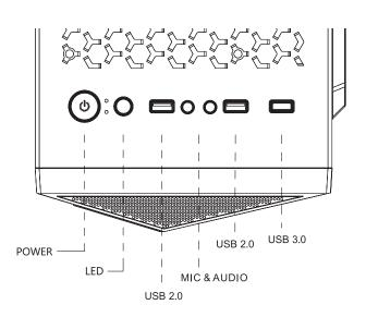
\*Long press LED Button 3 second for switching to RGB sync mode
