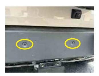
**Step 3:** Using the provided M6 Flat Head screws, vibratite, and your 4mm Allen tool, attach the bracket to your factory bumper. hand tighten with a 1/2 turn after.
