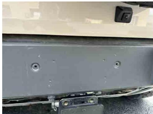
**STEP 2:** Take the included spacers, and place them behind the plate in the gap on each screw location where you will screw in the provided M6 flat head screws and the plate mount.
