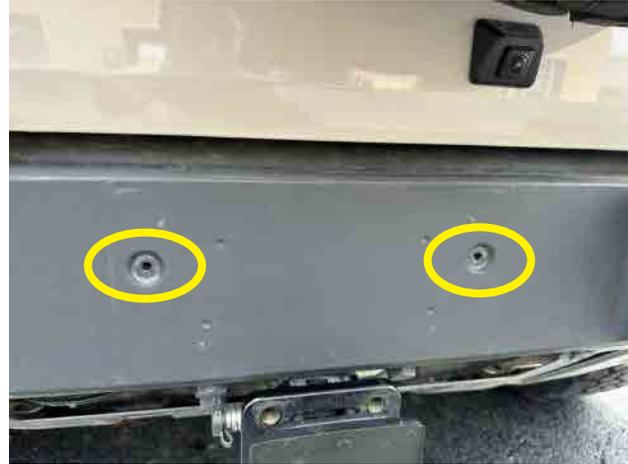
**Step 3:** Using the provided M6 Flat Head screws, vibratite, and your 4mm Allen tool, attach the bracket to your factory bumper. hand tighten with a 1/2 turn after.
