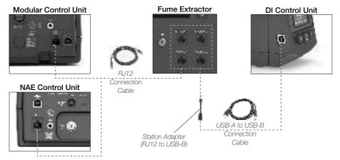
From software versions 8886887 (DDE,HDE) and 8886784 (NAE) on, the connected fume extractor can be configured and controlled through the Peripherals (1) menu of the control units. DI does not support this function.
