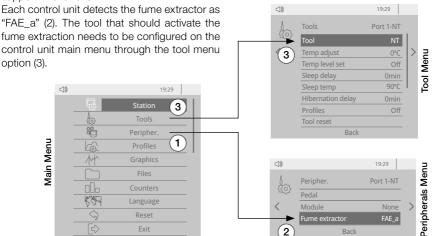
Connect up to 4 control units (connector FAE/ROBOT) to the fume extractor connectors (STATION 1, STATION 2, ...). Each tool connected to these control units can start and stop the fume extractor.
