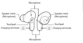
\*Make sure that the charging terminal is not soiled with foreign substance.
