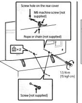
The length of the M6 machine screw differs dependin on the rope or chain diameter. Please refer to below
