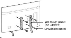
• If using an electric screwdriver, set the torque at approximately 1.5 N·m {15 kgf·cm}
