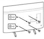
2 Attach the Wall-Mount Bracket (not supplied) using the screws (not supplied).
