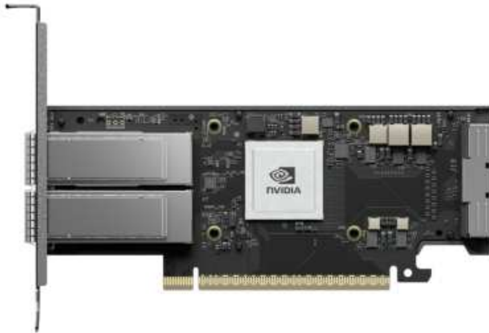
Figure 1. ThinkSystem NVIDIA ConnectX-8 8240 400Gbs QSFP112 2-Port PCIe Gen6 x16 Adapter (full-adapter gold case and heatsink removed)
