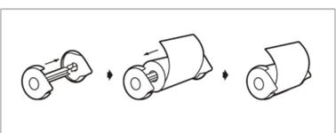
3. Place the paper roll into the printer and straightened the paper as shown in the picture above.
