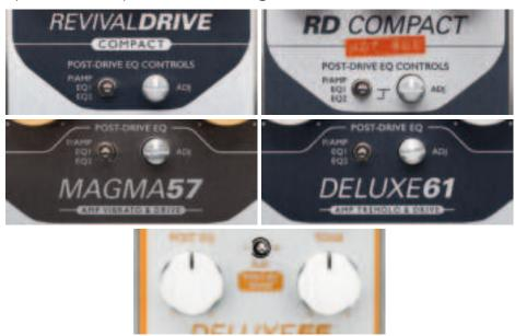
Move the POST-DRIVE EQ switch into the P/AMP position, this removes the pedal's output filtering and the ADJ / POST EQ control becomes inactive.
