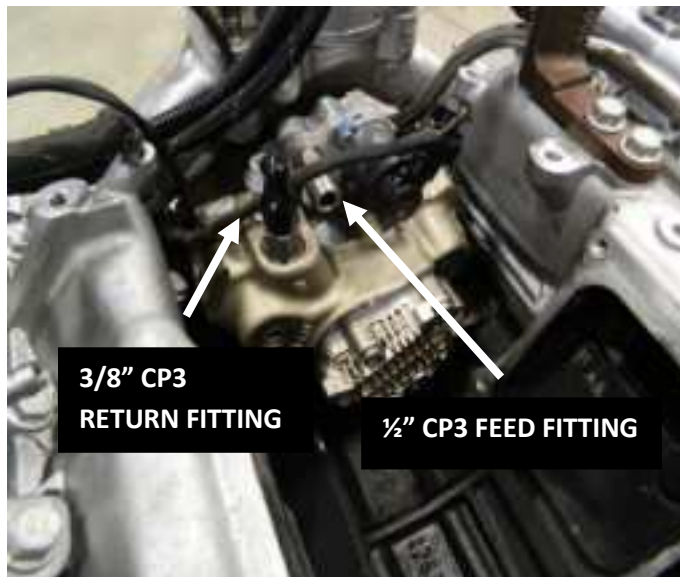
Fig. 11: Install the CP3 feed and return fittings
