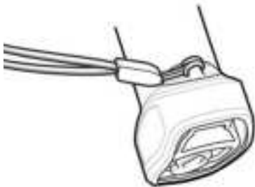
Figure 1-13 Insert Loop into Tether Point
