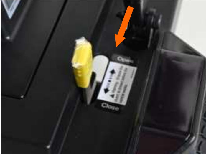
Fig 7.6.1 Drive Mode (Closed)
