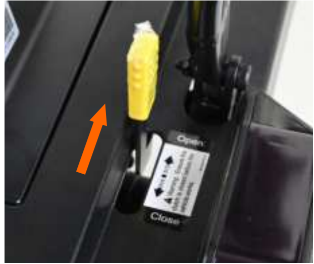
Fig 7.6.2 Freewheel Mode (Open)
