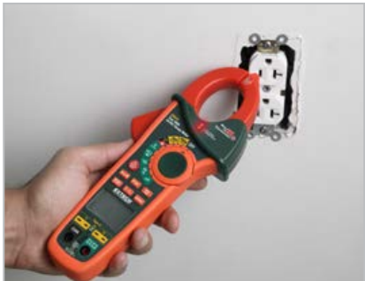
Non-Contact Voltage (NCV) Detection.
