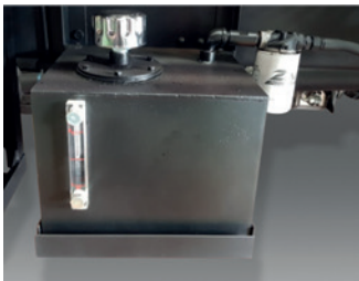
Oil tank Car Carrier HD120 / 260 Capacity : 46ℓ Note: Standard
