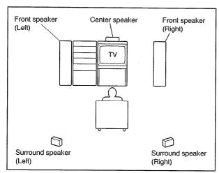
The sound reproduced by a speaker is easily influenced by such factors as room acoustics and the system's location in the room. Before finally deciding where the speakers are to be placed, please read the following information carefully.
