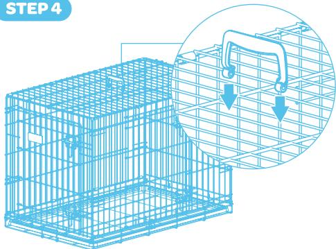
Repeat Step 3 on the other side of the crate. Attach handle to center top panel, as shown illustrated.
