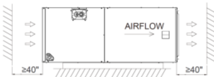
CLEARANCES IN THE HORIZONTAL POSITION
