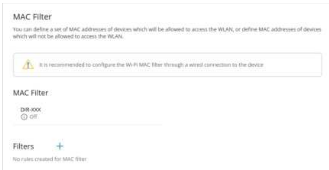
Figure 105. The page for configuring the MAC filter for the wireless network.
