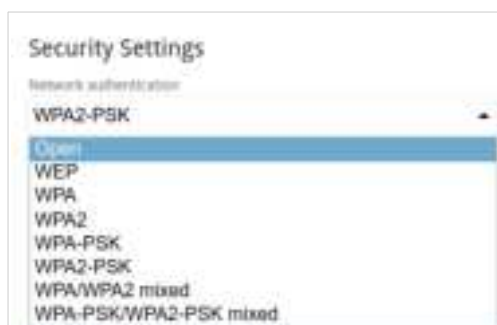
Figure 78. Network authentication types supported by the router.
