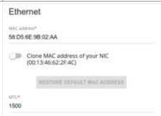
Figure 57. The page for creating a new Static IPv4 connection. The Ethernet section.
