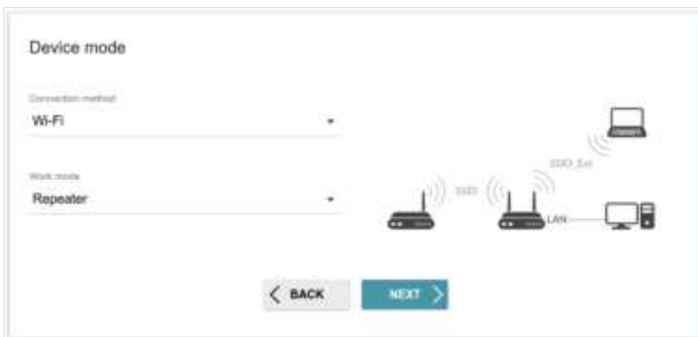
Figure 38. Selecting an operation mode. The Repeater mode.
