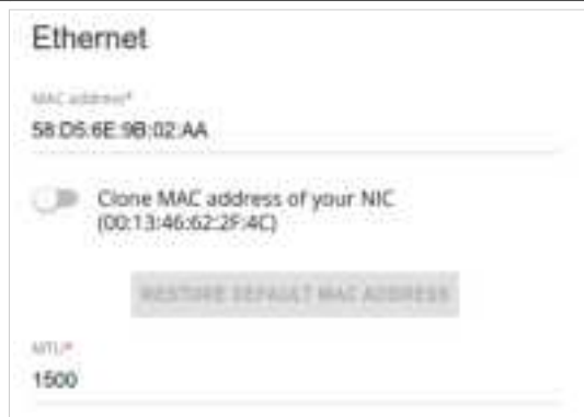
Figure 60. The page for creating a new Static IPv6 connection. The Ethernet section.
