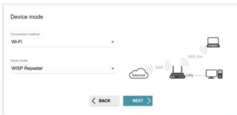
Figure 36. Selecting an operation mode. The WISP Repeater mode.
