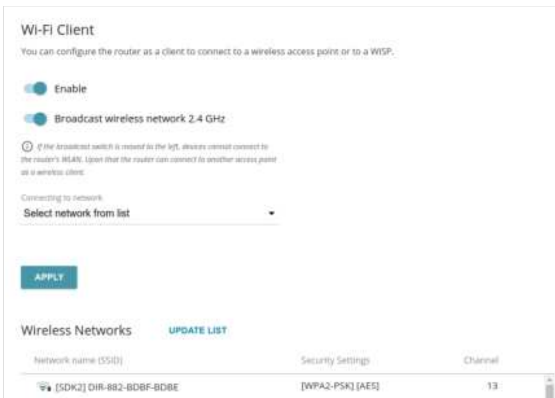
Figure 101. The page for configuring the client mode.
