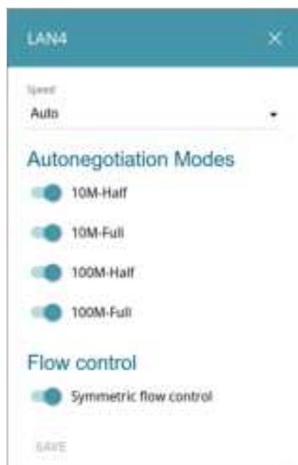
Figure 120. The window for changing the settings of the router's port.
