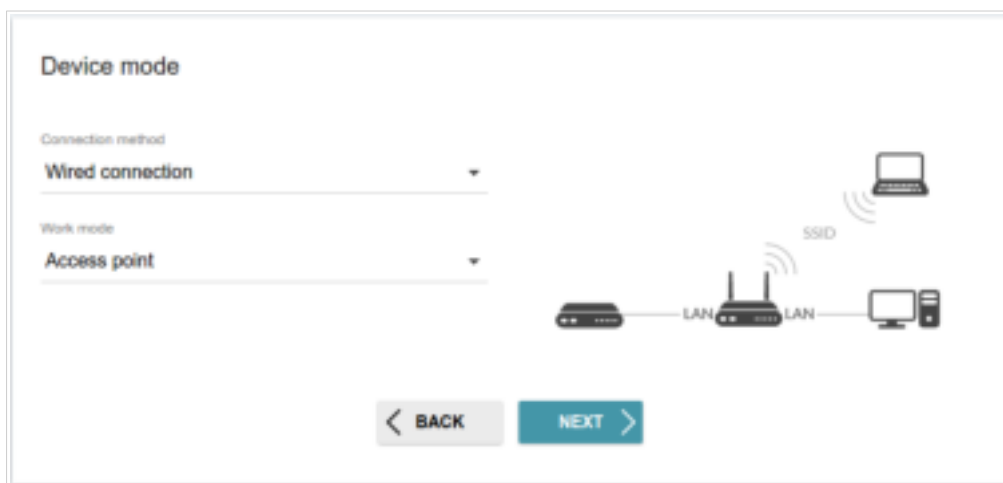
Figure 37. Selecting an operation mode. The Access point mode.
