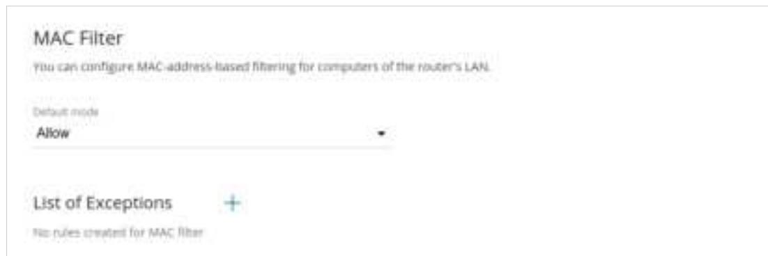
Figure 93. The Functions / Firewall / MAC Filter page.
