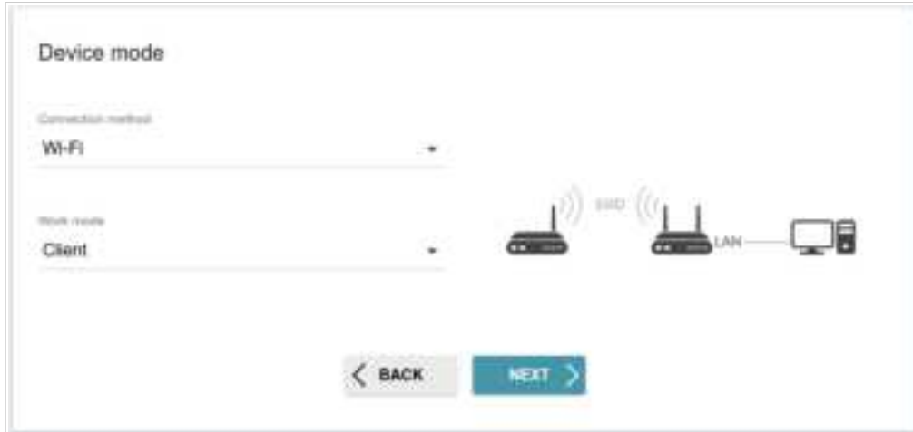
Figure 39. Selecting an operation mode. The Client mode.
