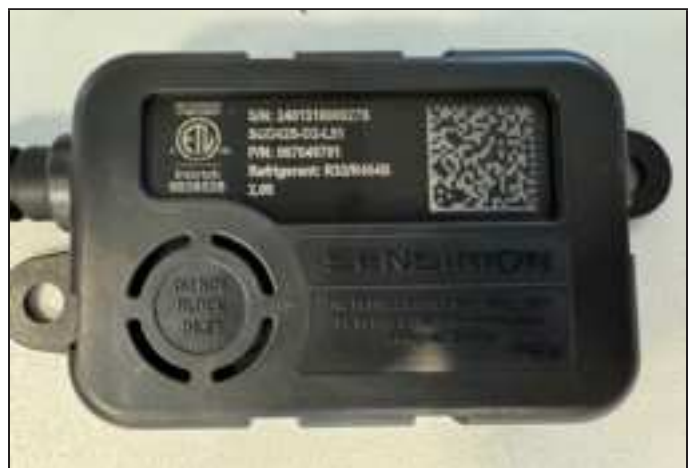
FIGURE 33. Example of Clear, Unobstructed Sensor Inlet
