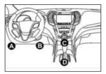
1.3 Plug the diagnostic cable into the vehicle's DLC socket.
