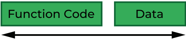
Fig.1 : MODBUS Protocol Data Unit
