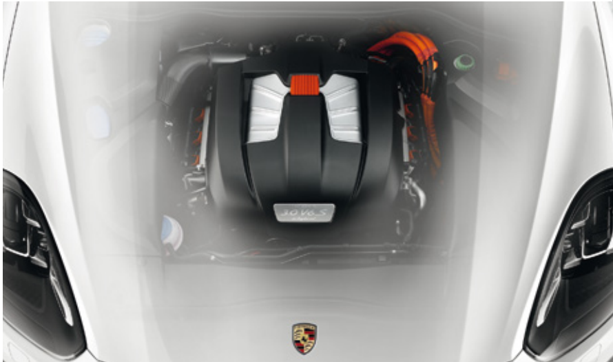
Cayenne S E-Hybrid (combined): 590 Nm between 1,250 and 4,000 rpm, 306 kW (416 hp) at 5,500 rpm
