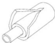
Pipe Wrap Insulation
