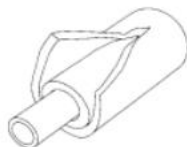
Pipe Wrap Insulation
