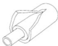
Pipe Wrap Insulation
