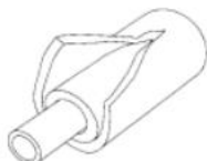
Pipe Wrap Insulation
