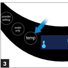
Press the "temp" button to select temperature.
