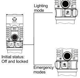
Rotate the Mechanicalswitch counterclockwise to turn on the lighting mode from the memory mode\*, then click the Clicky-switch to cycle through Eco-Low-Med-High modes.
