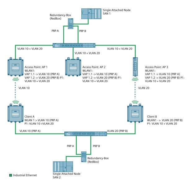
The access points (AP 1, AP 2 and AP 3) and the RedBox at the AP end are connected to each other via a switch. PRP network A und B are separated from each other via VLANs.
