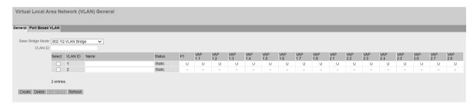
On this page you specify whether or not the device forwards frames with VLAN tags transparently (IEEE 802.1D/VLAN-unaware mode) or takes VLAN information into account (IEEE 802.1Q/VLAN-aware mode). If the device is in the "802.1Q VLAN Bridge" mode, you can define VLANs and specify the use of the ports .
