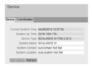
The boxes "Current System Time", "System Up Time" and "Device Type" cannot be changed.
