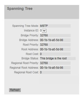
If Spanning Tree is turned on, the information about the status of the instance selected in the "Instance ID" drop-down list is displayed and the information about the configured ports is shown in the table. The information shown depends on the Spanning Tree mode.
