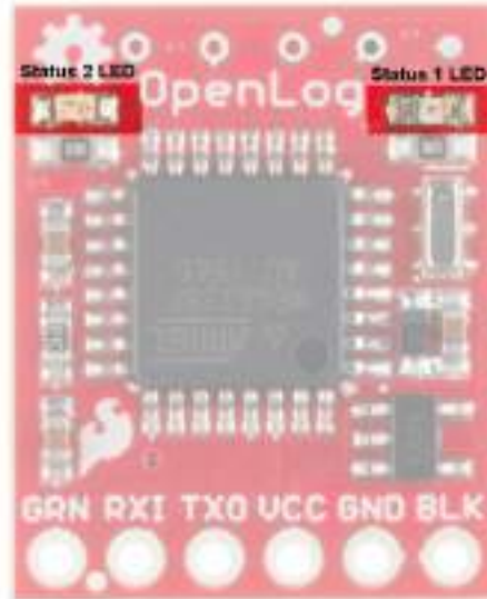
Status LEDs on the OpenLog.
