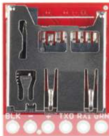
microSD Slot on the bottom of the OpenLog.
