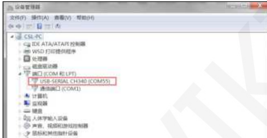
Figure 3 Identifying CH340 ports
