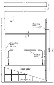
Note: dimensions in mm, tolerance +/- 2 mm
