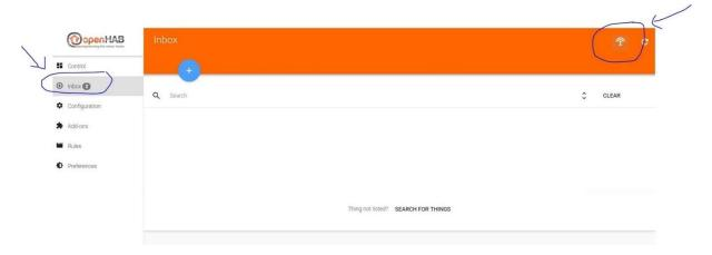
When you will call it, you have 60 seconds to add the device. It's easier to track the process in the logs. During this period, you need to follow Device manual to put it in Association mode. Sometimes you just need to give it power.
