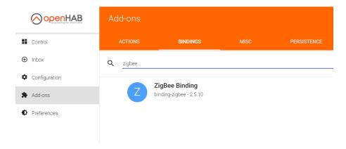
Once installed you can go to the **Configuration->Things** section of the menu and add new Thing. Select **Zigbee Binding -> Ember EM35x Coordinator** and then Configure it properly:
