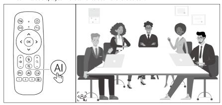
Step 2 Face the camera and make the "" gesture, a green frame will appear on the screen and frame the position of the gesture to select the person to be tracked. After the tracked person has been selected, the screen will display the "Presenter Tracking Active" prompt, indicating that tracking mode has been successfully activated (Note: Please release the gesture after tracking mode has been successfully activated).
