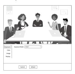
**Exposure Mode**: Full Auto, Manual, Shutter Priority, Iris Priority, Bright Priority, Smart. **ExpComp Mode** (Exposure Compensation Mode): On, Off (Effective in Full Auto mode).
