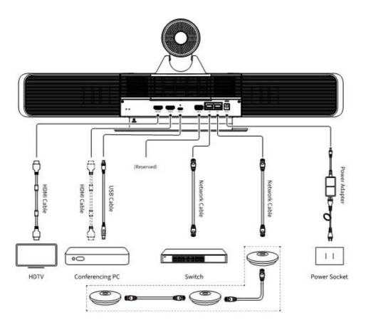
The recommended horizontal cascade distance is 3 meters, and the maximum number of cascades is 3 The EXT LAN port can power the extension microphones over PoE.
