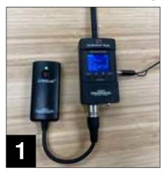
**1.** Connect your DMXcat or console to a Multiverse Node, or any other Multiverse wireless DMX/RDM transceiver.
