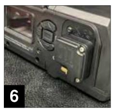
**6.** Attach the Multiverse Connect Module to the plug using the two screws from the fixture's plastic plate, ensuring it is securely connected.
