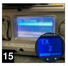
**15.** Navigate to the "DMX Universe" menu to confirm the selected universe matches the Multiverse Node, or other wireless DMX transceiver. In this example, Universe should equal 2 (refer to step 3).
