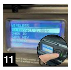
**11.** In the "Wireless" menu, the fixture will auto-detect if it is connected to a Multiverse Connect Module.
