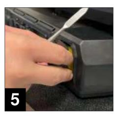
**5. Remove the plastic plate** from the base. This exposes the Universal Connect Module plug.
