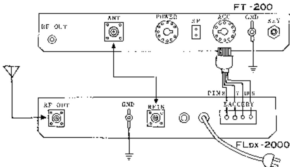
Diagram shows correct connections for using the FL DX 2000 Linear Amplifier with the FT-200.
