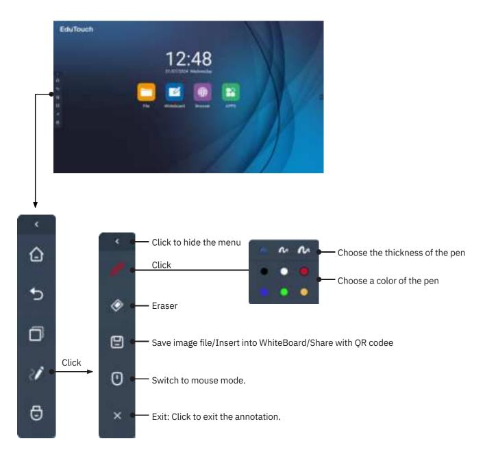
Note: In annotation mode, it supports Gesture Eraser function. (When the screen area is sufficiently touched by the hand, the wipe icon appears, move the icon to wipe.)
