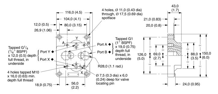
◆ See "Mounting Surfaces" section above for port usage.
