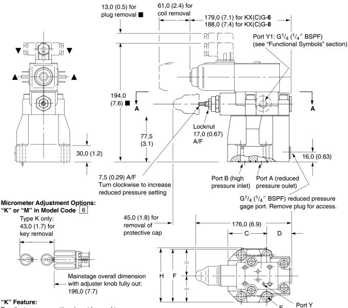
To adjust pressure setting, insert key and turn clockwise. Turn micrometer knob clockwise to increase pressure setting; counter-clockwise to decrease setting. When the key is removed the knob can spin freely without affecting the pressure setting.
