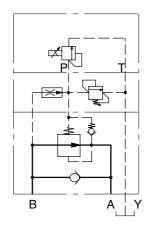
Manual Pilot Drained to Port Y; Electrical Pilot Drained to Port Y1◆: Model Code 8 = 3 Symbol for KXG models. For KXCG models add check valve symbol and internal connection A-B.
