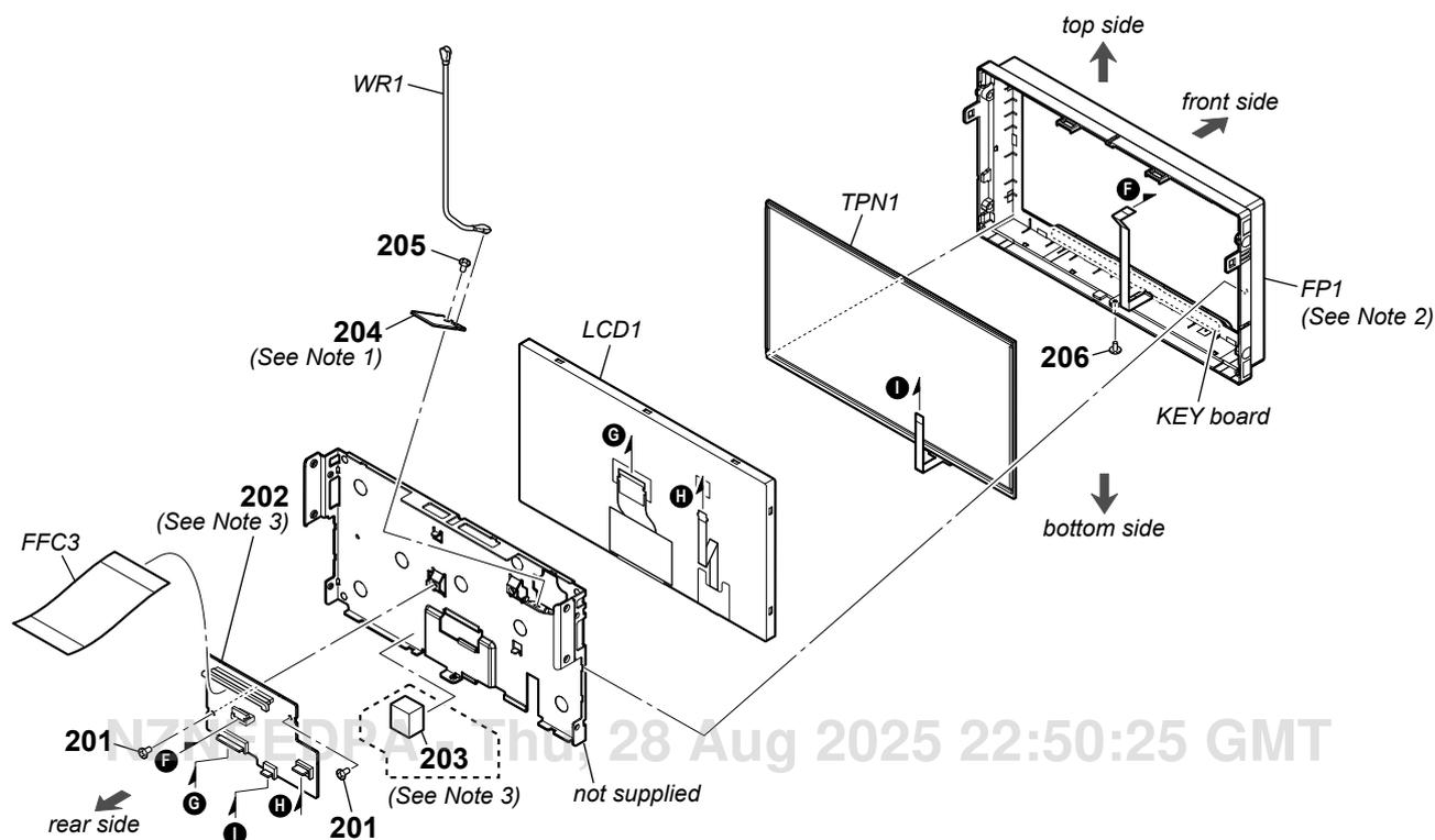
**Note 1:** When the complete ANT board (Ref. No. 204) is replaced with a new board, or the ANT board is repaired, be sure to refer to “IMPORTANT NOTE OF REPLACING THE ANT BOARD” on page 8, and perform it.
