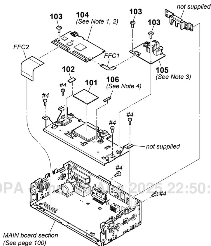
**Note 1:** Replaced old complete SoM board (Ref. No. 104) is destroyed with the hammer, and dispose it.
