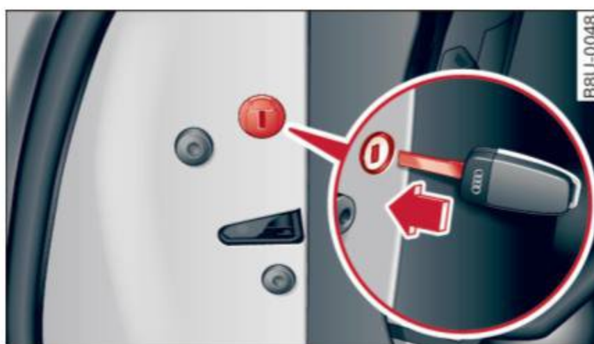
Fig. 20 Front passenger's door/rear doors: emergency lock
