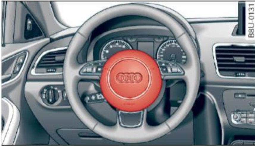
Fig. 112 Location of driver airbag: in steering wheel
