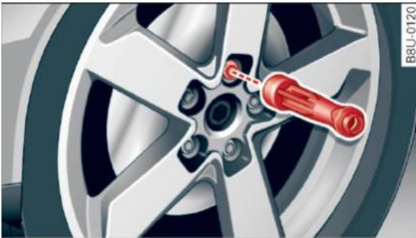
Fig. 154 Changing a wheel: using the hexagonal socket (with the blade removed) to turn the bolts
