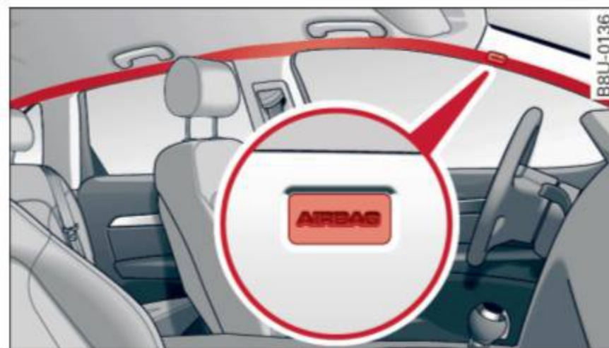
Fig. 118 Side curtain system, driver's side: side curtain airbag location
