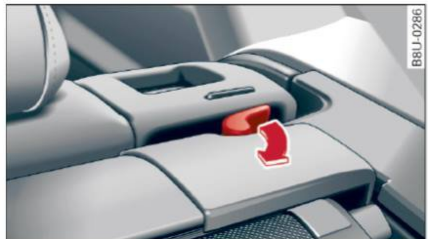
Fig. 56 Right front section of the luggage compartment: removing the luggage compartment cover
