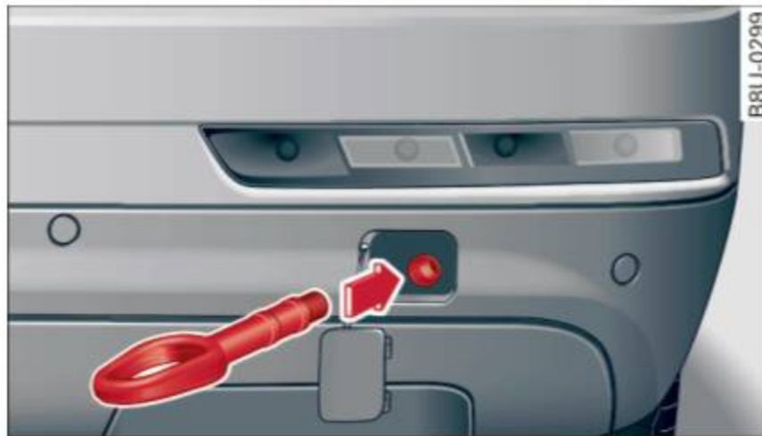
Fig. 165 Rear bumper: installing the towing loop
