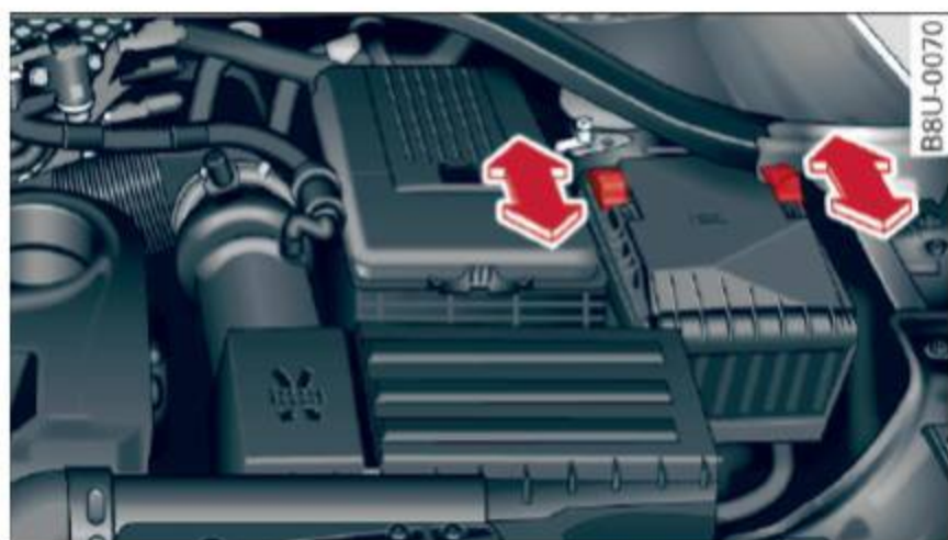
Fig. 159 Engine compartment: removing the fuse panel cover
