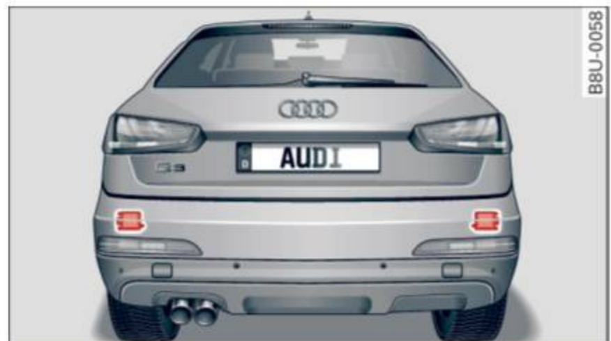
Fig. 82 Rear of the vehicle: position of the sensors
