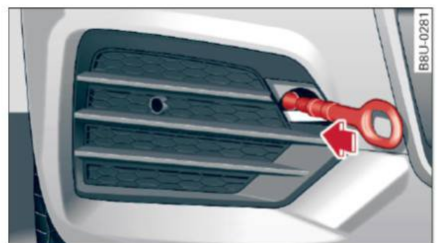
Fig. 163 Front bumper on the right side: screw in the towing loop
