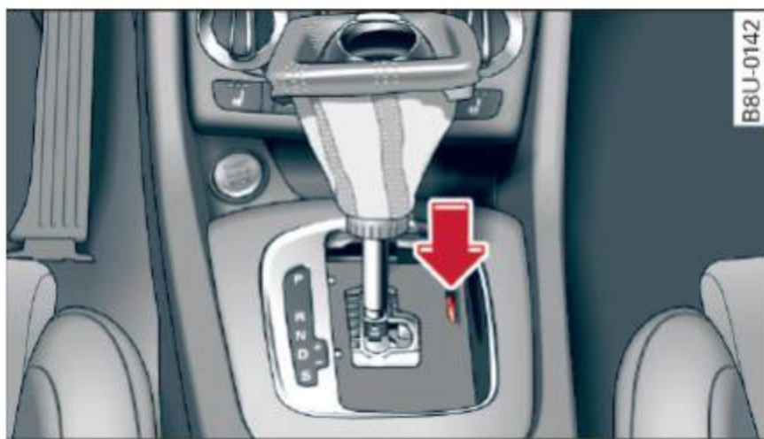
Fig. 77 Selector lever: emergency release
