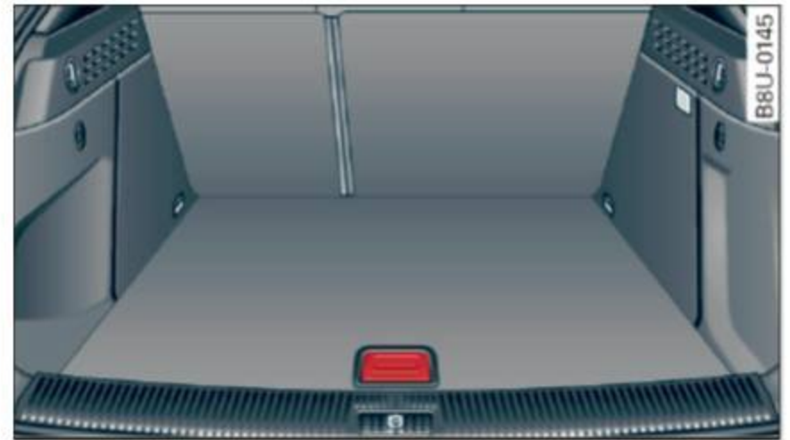
Fig. 63 Luggage compartment: reversible cargo area floor with the decorative side facing up
