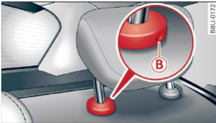
Fig. 50 Rear head restraints: release point
