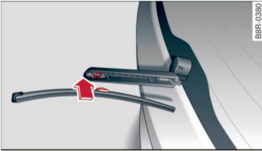
Fig. 42 Rear window wiper: removing the wiper blade
