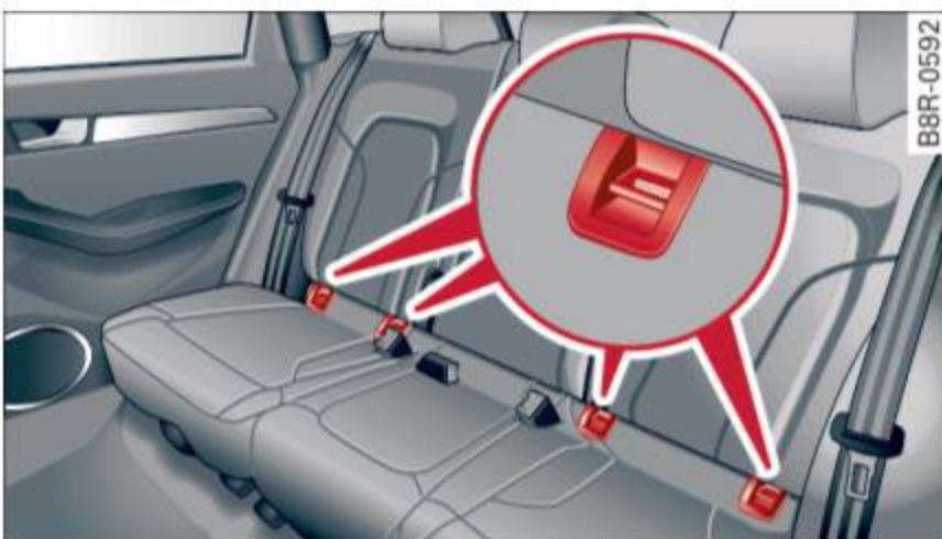
Fig. 127 Rear seats: lower anchorage bracket locations
