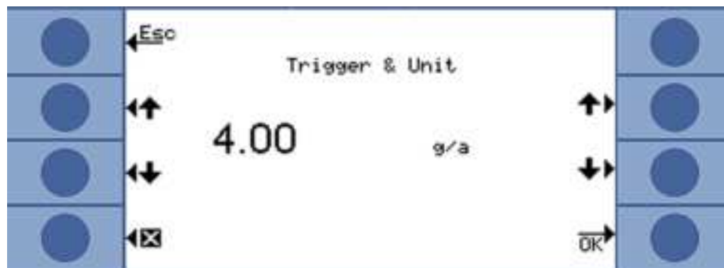
Fig. 22: Setting trigger value and unit
