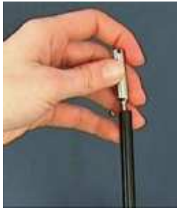
Fig. 7: Screw water protection tip on tight
