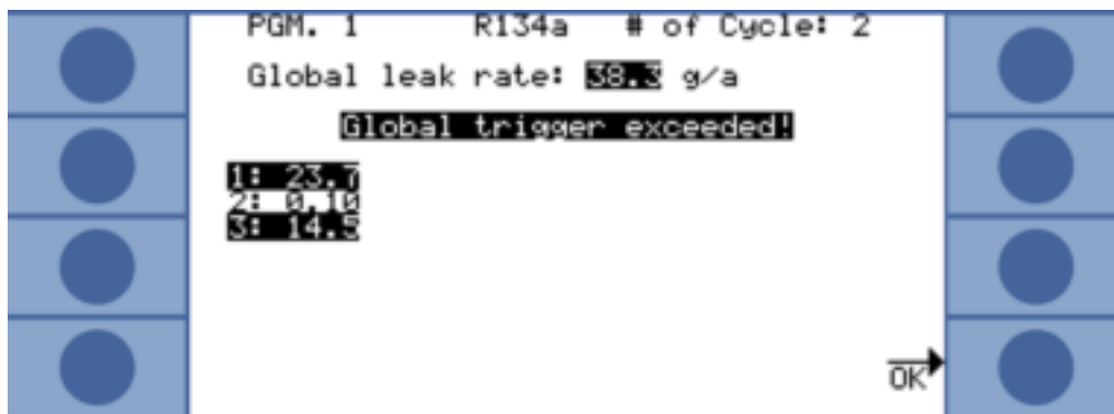
Fig. 37: Search with I•Guide-Program 1 for gas R134a: The trigger value and the total leakage rate were exceeded at measuring points 1 and 3.
