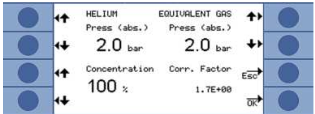
Fig. 27: Setting the parameters for gas equivalent and diluted gas
