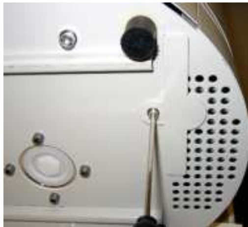
Fig. 47: Loosening the air filter cover
