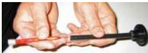
Fig. 6: Pushing out the capillary
