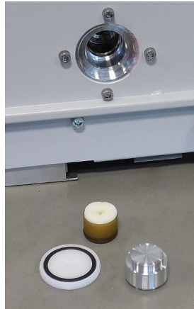
Fig. 49: Operating fluid reservoir open
