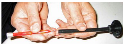
Fig. 6: Pushing out the capillary
