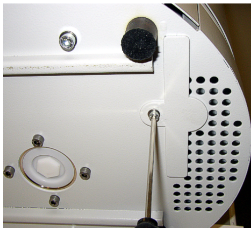
Fig. 47: Loosening the air filter cover
