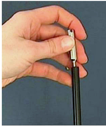
Fig. 7: Screw water protection tip on tight
