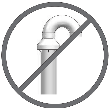
Figure 5-5 Do Not Install U-Bend to Rain Cap
