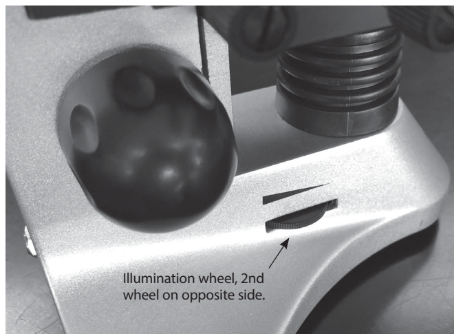
Figure 5. Focus knob, illumination wheel, and bottom illuminator shown
