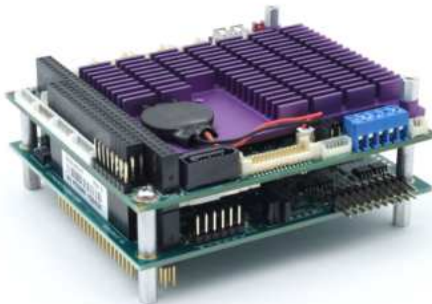
Figure 1-3: Samson with PC/104 I/O module installed underneath
