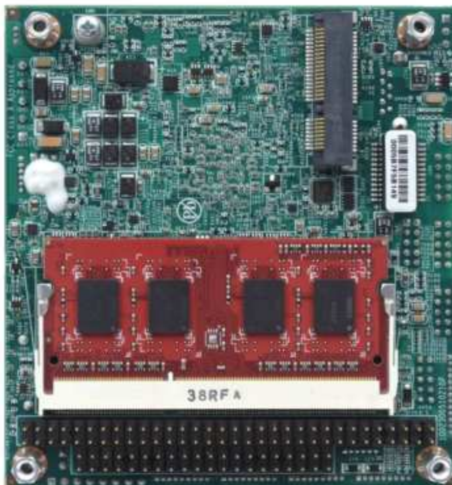
Figure 1-2: Samson PC/104 SBC – Bottom View with SODIMM RAM
