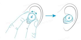
**Step 4:** Take the Fit Test on the soundcore app to check if the ear tips are the optimal size and to ensure the earbuds are sitting in the perfect position.
