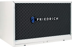
Standard Grille Premium, stamped steel grille with powder coat paint. Ships with WSE sleeve. Galvanized steel inner and outer weather panels also ship with sleeve.
