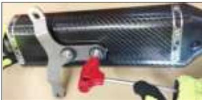
**ENG** Fix the support bracket to the silencer, using the two hex head screws M8x35 with 8x24 washers, in the pack, making sure to position the aluminum spacers in contact with the silencer ; tighten the screws.
