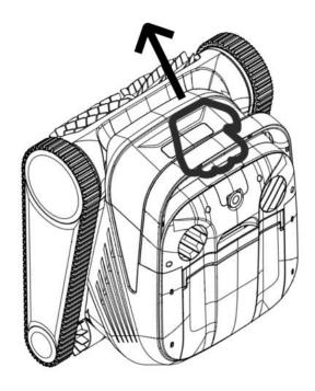
11) After cleaning cycle, open the filter cover, lift the basket, clean the filter basket.
