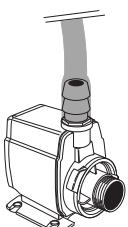
Slide the hose (8) onto the hose connector (9).
