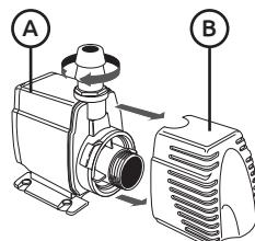
Remove the filter cover (B) of the pump, it is not necessary with a marine aquarium.
