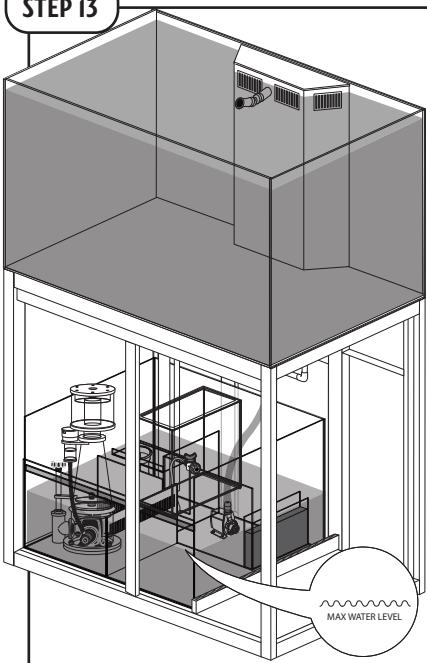
Open the tap of the transit pipe and fill the tank until the maximum water level has been reached in the sump.
