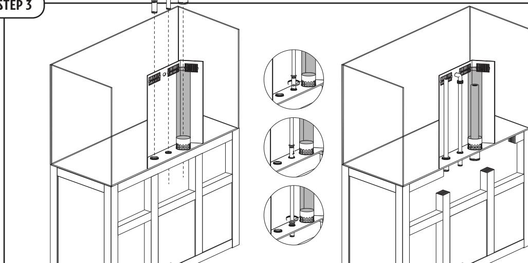
Place the transit pipe (1), the outflow pipe (4) and the overflow pipe (6) in the slots.
